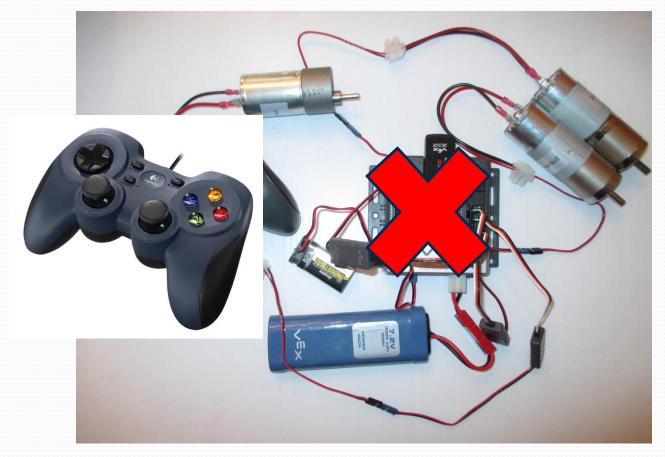
VEXnet joystick replaced by Logitech F310 Joystick/Controller
